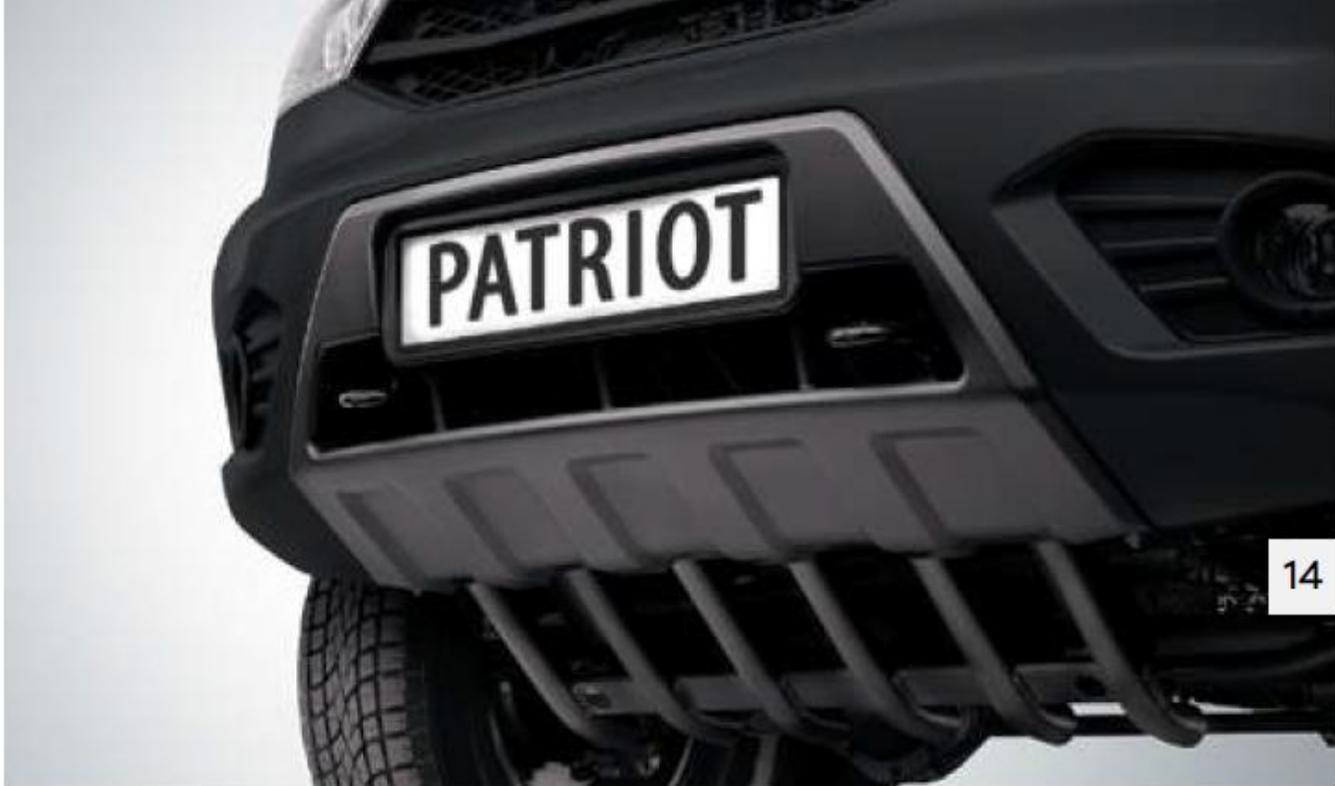
Critical parts of the vehicle demand solid protection, because collisions with obstacles are part of the very nature of the powerful UAZ Patriot. The transmission, transfer case, steering rods and fuel tank should all be well protected. The protection of steering rods is necessary for their safety and proper operation when encountering rough terrain and obstacles. We offer two types of protection: steel pipe or sheet steel skid plates.
