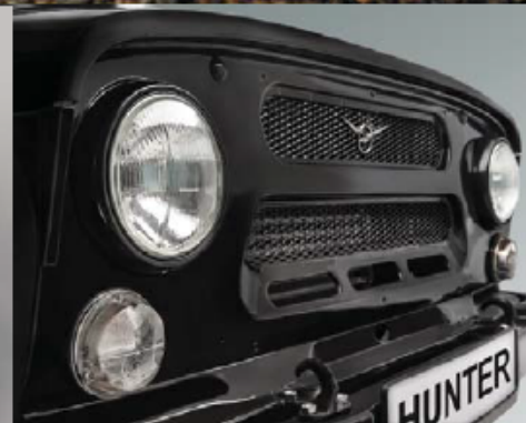
A metallic fine mesh grille protects the radiator from aggressive environment
