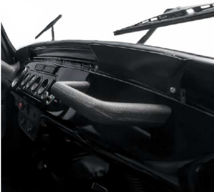
A handle for easy getting in and out of the front of the cabin
