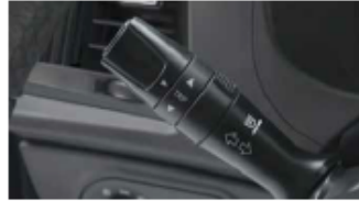
Left-hand steering column control with turn signal indicator and on-board computer control
