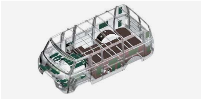
Improved vibration and noise insulation package all over the body, and special body-mounted pads
