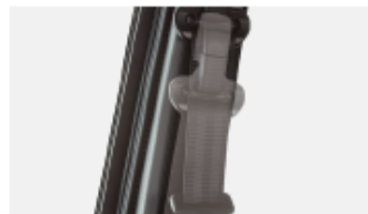
Front safety belts with tensioners, force limiters and new height adjusters
