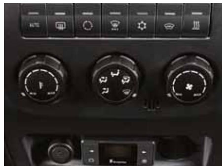
Air-conditioning and heating control unit
