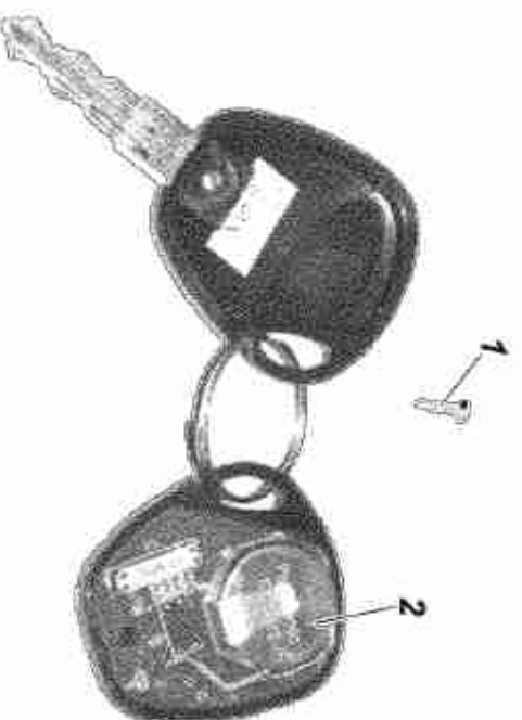
Fig. 3.15. Remote control panel: 1 — screw; 2 — replace battery
